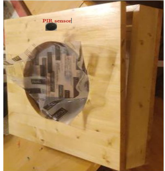
Smart window with PIR sensor placed outside
